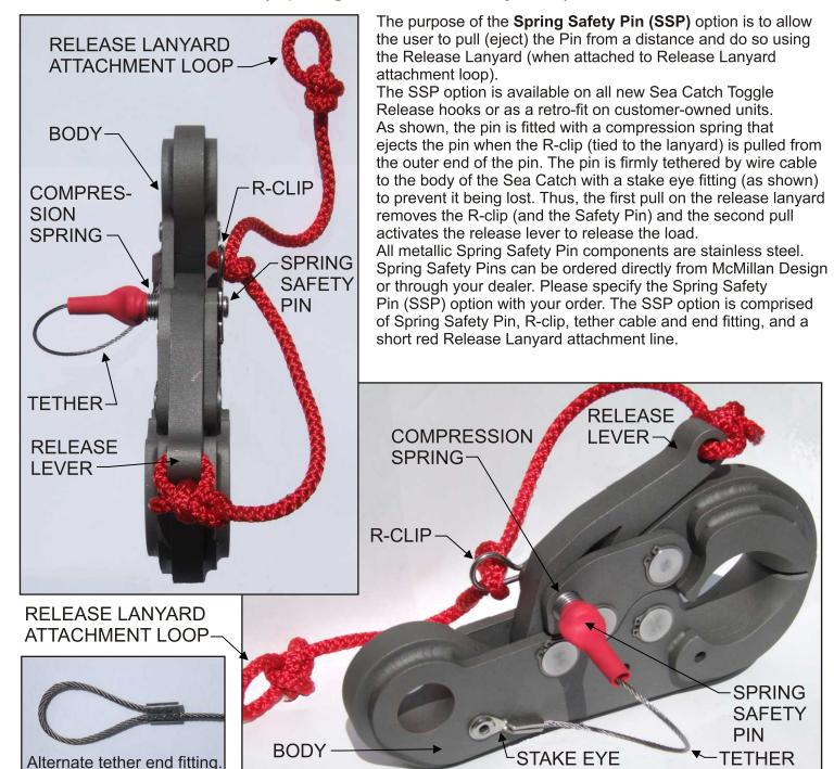
TIPS: The Release Lanyard is never to be used as a tag line. Doing so may cause the R-clip to be pulled inadvertently and rendering this safety measure ineffective. Rigging the Spring Safety Pin as shown using the Release Lanyard rather than a separate line dedicated to the R-clip, prevents the Release Lever from binding the Spring Safety Pin and pre-
